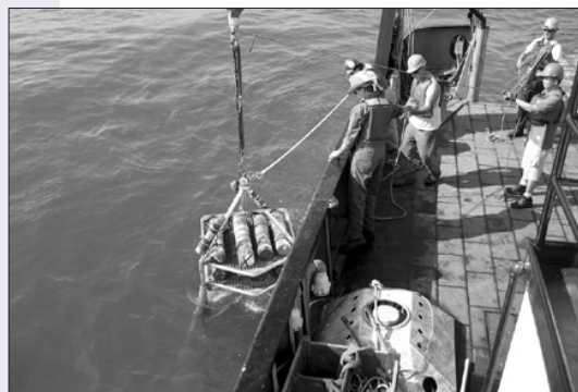
A tripod outfitted with computers that control acoustic instruments is lowered to the ocean floor to measure water flow and sediment processes. Photo: University of South Carolina
